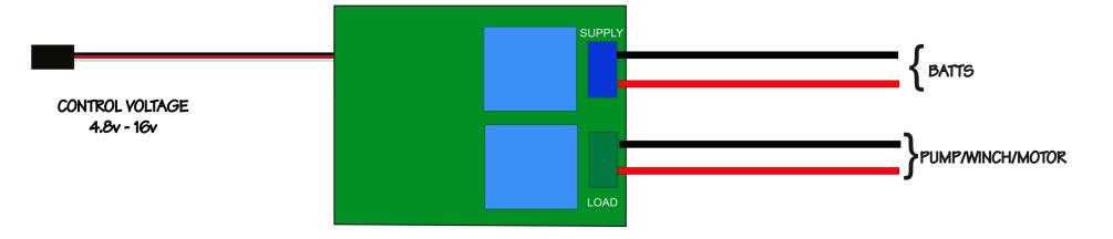
PLEASE ENSURE UNDERSIDE IS ADEQUATELY PROTECTED FROM ANY CONDUCTIVE SURFACES WHICH MAY SHORT CIRCUIT THE COMPONENTS
